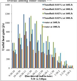
**Fig: 1.** Experimental variation in useful heat gain by nano fluid and water at different conc and volume flow rates [15]
