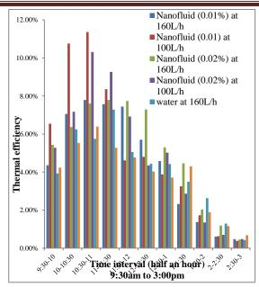
**Fig: 3.** Experimental variations in overall thermal efficiency for different fluids
